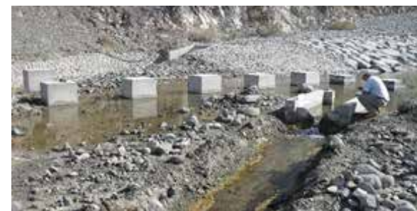
Measuring see page at the V-Notch downstream of Sifuni Dam
